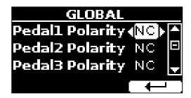
By [DATA/ENTRY] or [< >] buttons select "NC" value to set the switch pedal as "Normal Closed" working, select "NO" value to set the switch pedal as "Normal Open" working.
