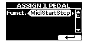
Any time you press the controller assigned to the "MidiStartStop" function, you send the Start (FA) and the Stop (FC) midi command via midi to an external device.
