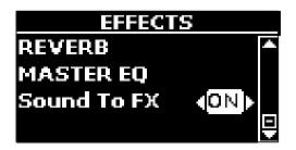
Setting the "Sound to FX" parameter to "ON" the last setting of FX-A, FX-B and FX-C of all parts is frozen when the sound changes.
