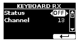
By [DATA/ENTRY] and [<>] buttons select the "Status" value field and set it to ON to activate the MASTER RX remote keyboard channel function.
