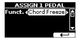
By [DATA/ENTRY] or arrows buttons select the CONTROL environment and select one of the available assign pedals controllers. By [DATA/ENTRY] or arrows buttons select the "Chord Freeze" function.
