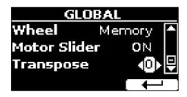
Press [MENU] button on panel, by [DATA/ENTRY] or arrows buttons select GLOBAL environment and choose "Transpose" to edit the value of this parameter.
