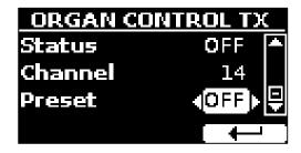
By [DATA/ENTRY] and [<>] buttons select the "Status" value field and set it to ON to activate the transmission of Organ midi channel.
