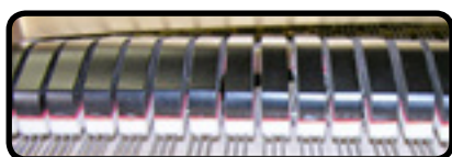
(C) "DAMPER" pedal is released, felt dampers are resting on strings.
