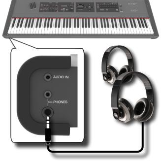
**2.** Rotate the VIVO S7/S3's [VOLUME] knob to adjust the volume of the headphone.
