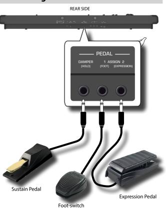
**1.** Connect to the DAMPER (HOLD) socket a sustain pedal.
