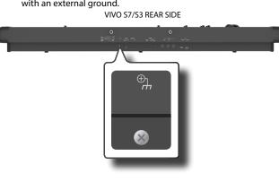
**1.** Use the screw-type ground terminal to connect to ground or to connect to the chassis of the mixer, preamp, or other device in your system.
