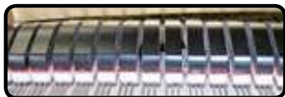
(C) "Forte" pedal is released, felt dampers are resting on strings
