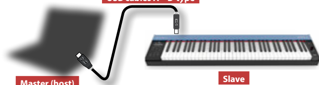
Basic USB system architecture
